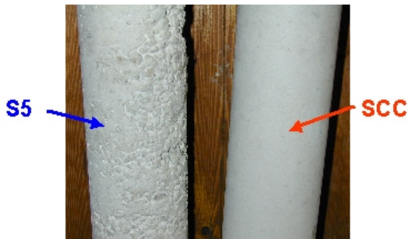
Fig. 1 – Skin effect marble-like of SCC with respect to a traditional concrete at a superfluid consistency (S5), both placed without compaction.
