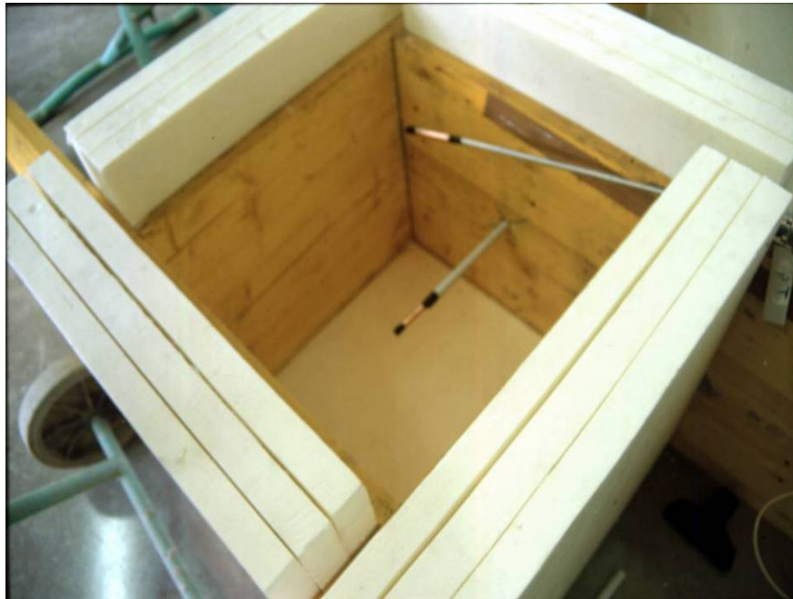
Figure 16 – Semi-adiabatic test to simulate the placing of a layer of slab.
