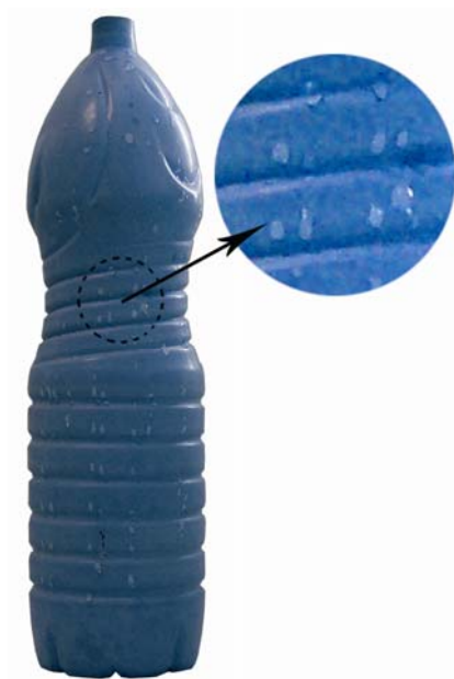
Figure 4 Colored SCC placed into a plastic bottle and then demoulded. Note on the right the drops of water not absorbed by the concrete skin.
