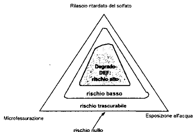
Fig. 1 - A holistic model showing DEF-damage as a function of late sulfate release, microcracking, and exposure to water (11).
